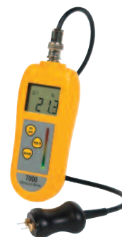
Measures moisture in concrete / hard floors
