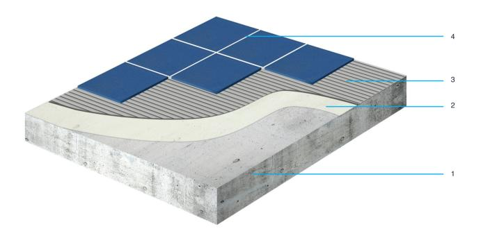
\*Allow at least 6 weeks for structural concrete floors to cure and further 3 weeks for subsequently applied screed. In the event that a rapid setting cement replacement is used the drying time of screed will be greatly reduced. Contact the Technical Team for further information
