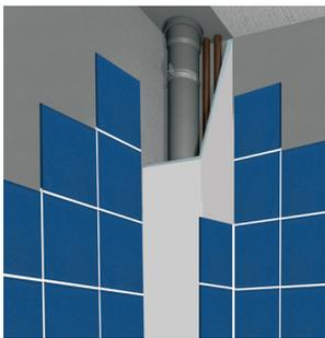
Smooth, paintable pipe covers are a quick and effective solution for hiding away unsightly pipework, simply choose the correct cover size and cut to length. Run a bead of Nicobond PU Adhesive along the 2 leading edges and press firmly into position.
