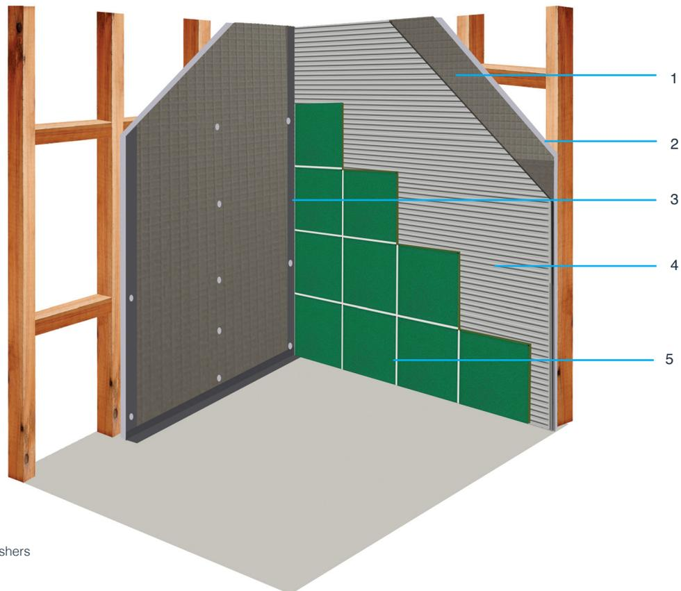
1. Screw board to stud work using Nicobond Galvanised Screws & Washers, taking care to screw down until the washer bites into the board. For boards less than 20mm thick, vertical studs should be set at 300mm centres. For greater thicknesses 400mm centres are suitable.
