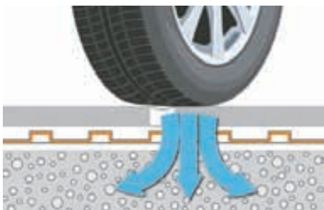
Transfers dynamic and static loads direct to the substrate.
